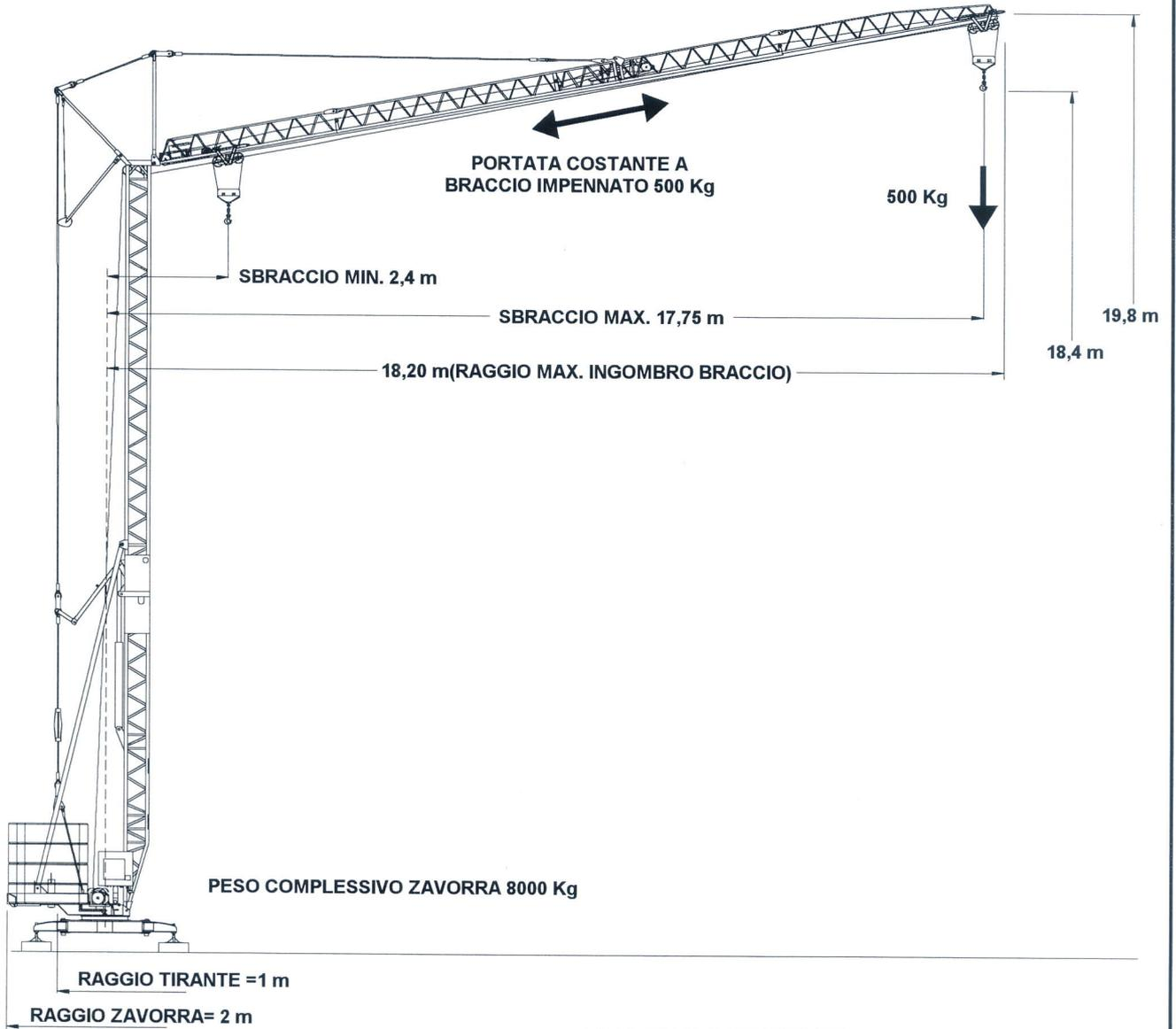
**DIAGRAMMA PORTATE CONFIGURAZIONE A BRACCIO IMPENNATO**
